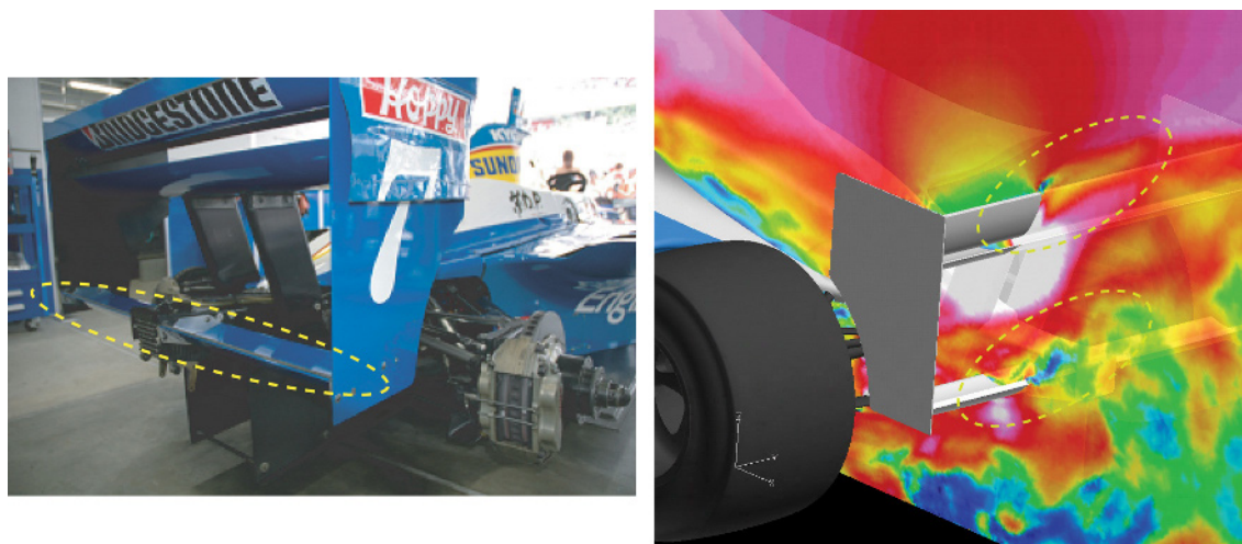
Fig. 9. The Gurney flaps on the trailing edge of a rear wing (left) and the flow reproduced by HPC-LES (right).
